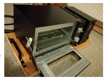
As for now I am still finding the right PID adjustments. The pcb's and solder paste are already waiting for the first run. © Well exiting...
