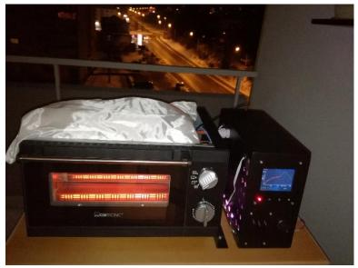
First test run on the balcony. The white stuff is original glasswoolinsulation. As I said, I left it off when I closed the toaster.
