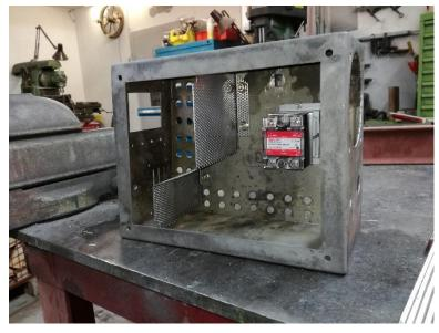
The picture shows the sheet metal box, with all the different holes for mountings and air vents.
