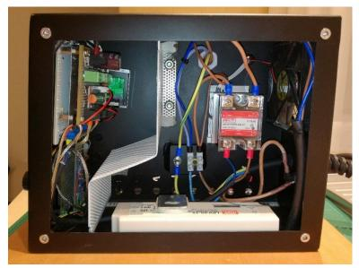
All the wiring in place. I added a 10A fuse, seen bottom right, with the two brown cables connected to it.
